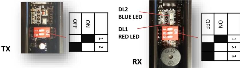
1. Set the TEST DIP 1 of the TX motherboard to ON.
