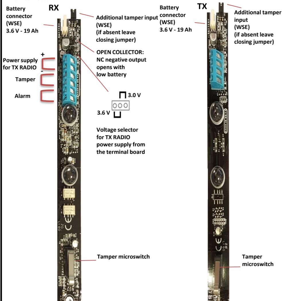
The tamper output in the terminal board is closed if both columns have their own microswitches closed.
